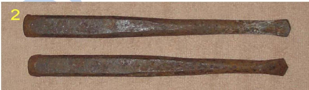
Typical Plug Drills - (Top) drill with a round blade (bottom) drill with pointed blade
