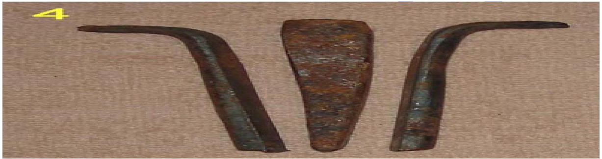
Two feathers (shims) with a plug (wedge) between them
